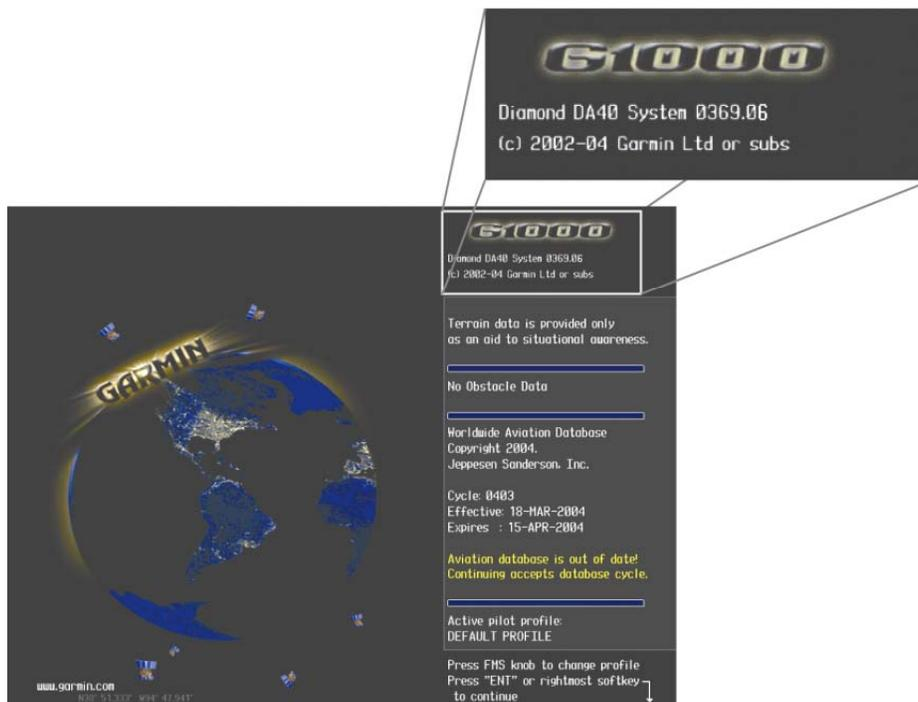
2. This ‘System’ number is the System Software Version. It correlates to the G1000 SW Loader Card used to load the software to the system:
