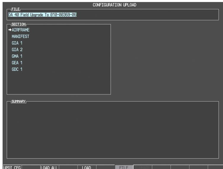
1. Go to the Configuration Upload page using the small FMS knob.
