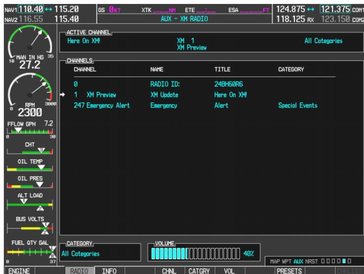
2. Using the channel control located in the cabin, verify that you can increment and decrement the channels (the white arrow to the left of the channel list indicates the currently selected channel). Select channel 1 when complete.
