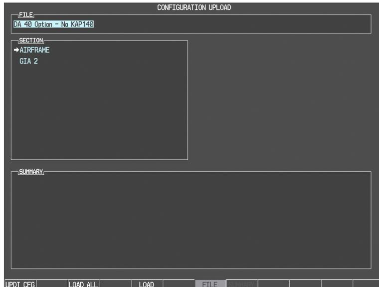
1. Go to the Configuration Upload page using the FMS knob.
