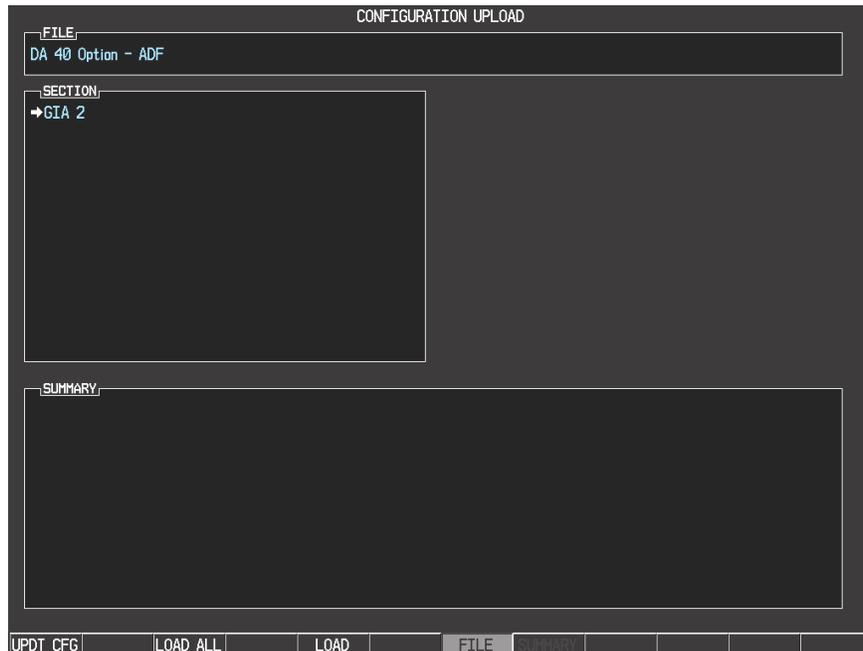
10. Go to the Configuration Upload page using the FMS knob.
