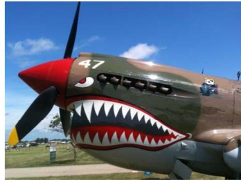
Appropriately known as “Stub Stacks” these simple metal tubes with minimal bends and no internal obstructions fulfill that primary purpose admirably well. So well, in fact, that when measuring the output of an engine to determine its horsepower rating, most manufacturers and testing facilities will use what they refer to as “Neutral” or “Test” Stacks (which are really just straight “Stub Stacks” with a standard length of 4”).
