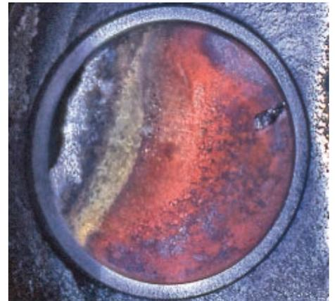
head's large thermal mass and dissipated through its cooling fins (see Figure 2). This "heat sink" arrangement is absolutely essential to the survival of the valve. Without it, the valve face would overheat and self-destruct quite rapidly.
